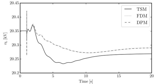
**FIGURE 7** Rotor angular speed of a synchronous machine (top panel) and voltage magnitude at a load bus (lower panel) of the All-Island Irish Transmission System (AIITS) following the outage of the largest in-feed [76]
