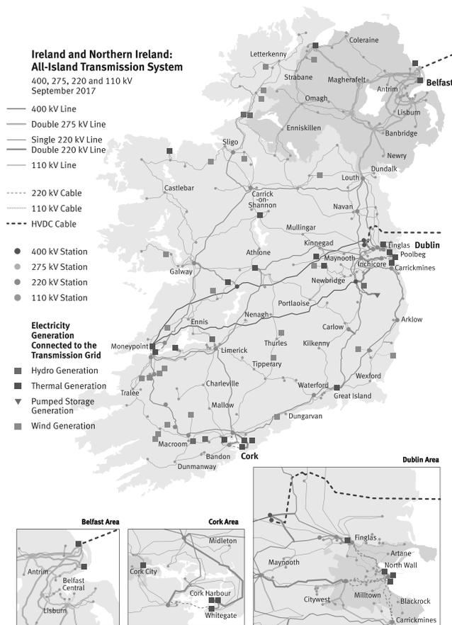
**FIGURE 5** Scheme of the All-Island Irish Transmission System (AIITS) (courtesy of EirGrid Group, available at [www.eirgridgroup.com](http://www.eirgridgroup.com))
